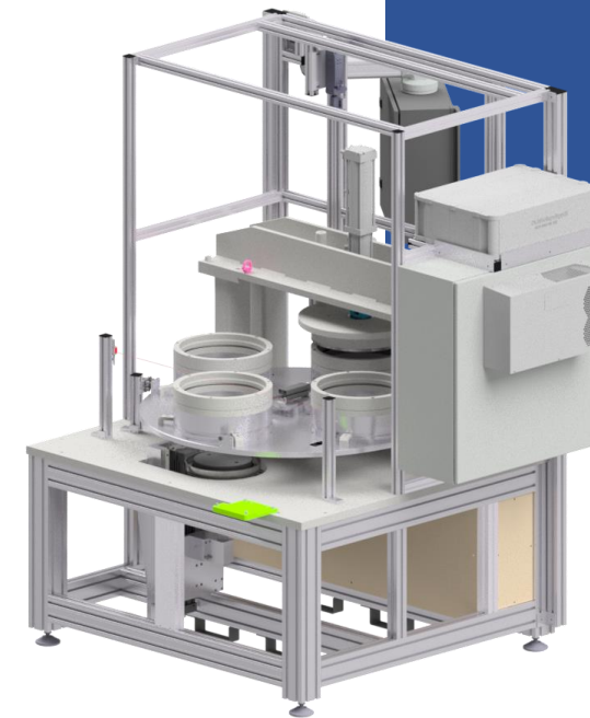
Leak testing machine as a rotary transfer system
